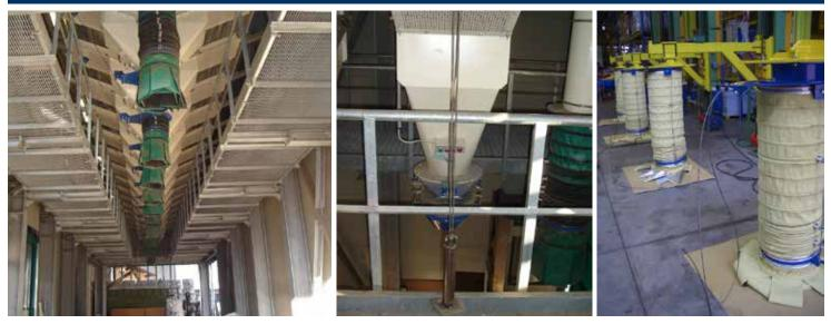
ZN Loading Bellows are used for efficient discharging of powders or granular materials into tankers.
