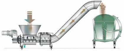
Screenings fall into the compactor hopper from which a rotating shafted spiral conveys solids to the compacting zone where they are dewatered and, at the same time, conveyed to the outlet. The compacting zone is equipped with spray nozzles for washing organic matter contained in the screenings. The liquid produced by washing and compacting is transferred back to the purification process through the screening channel.
