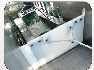
Self-adjusting grease scraper with limited water removal
