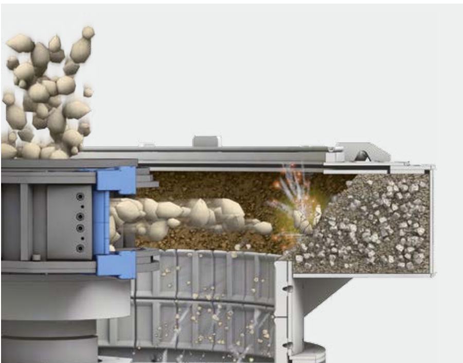
Functional principle with rock shelf (side view)
