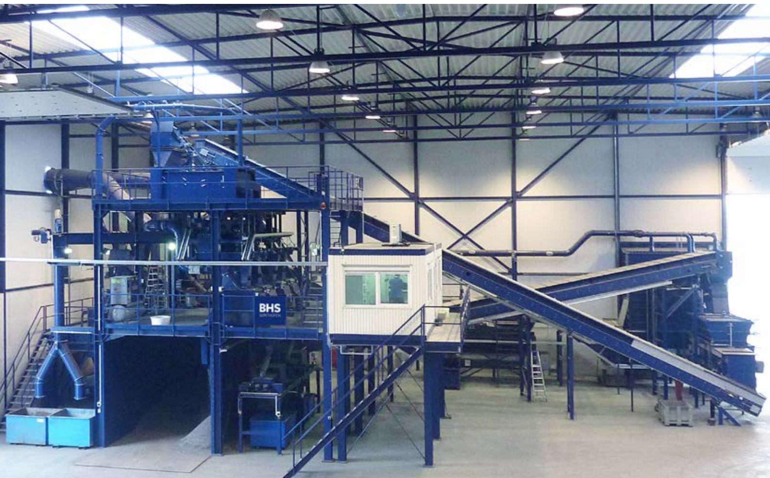
Fine treatment of shredder residue fractions with RPMV 1513
