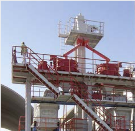
Two RPM 1513 for the production of dry mortar sand (0 - 1.6 mm) from limestone (8 - 20 mm)
