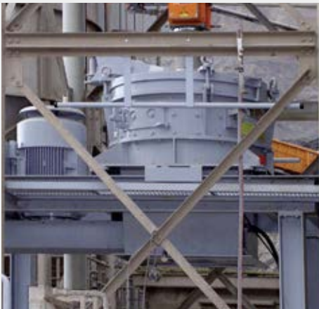
RPM 1113 for the production of high-grade crushed sand (0 - 2 mm) from off-spec gravel fractions (2 - 5 mm, andesite)
