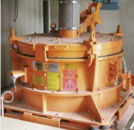
RPM 1113 for the production of concrete sand (0 - 2 mm) from gravel (16 - 32 mm)
