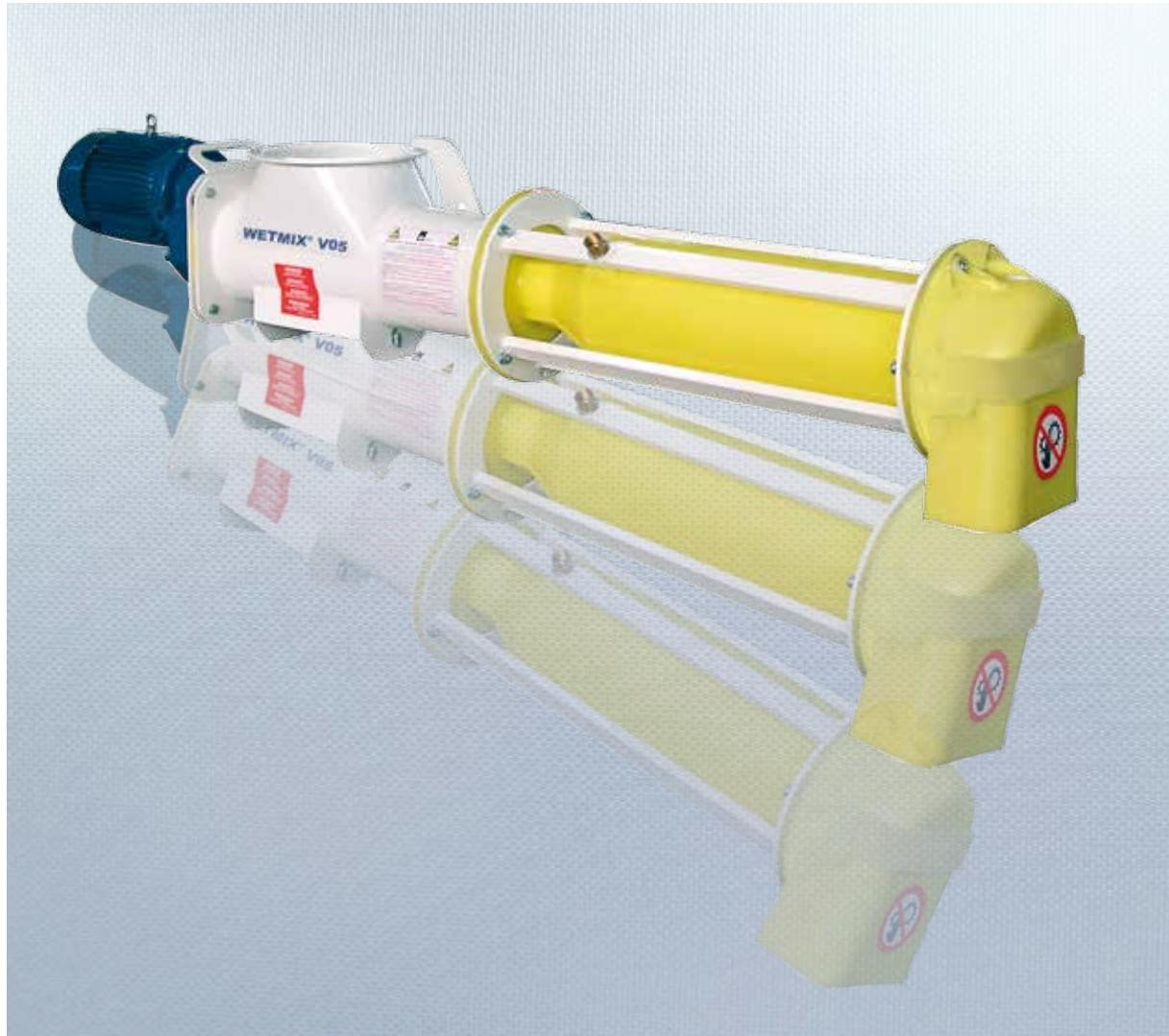
WETMIX™ V05 is a continuous horizontal single-shaft mixer with a mixing chamber completely manufactured from wear-proof SINT™ engineering polymer. Fitted under a small building site silo, it is used for the preparation of premixed mortars or plasters, directly on site.
