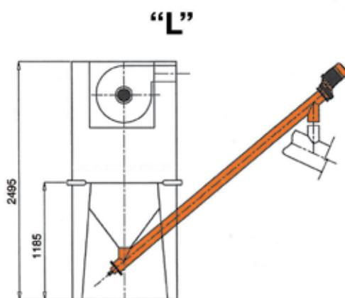
Version with inclined screw ( $l = 3000/5000$  mm)
