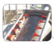
Rotary drum with cleaning nozzles
